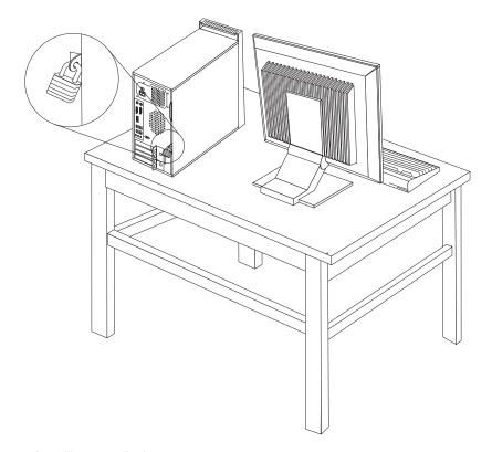
Figure 41. Installing a padlock
